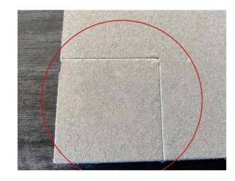
The cutting depth is adjustable, which can replace the die-cutting machine, saving time and labor.
